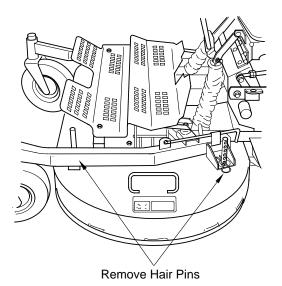
Figure 4-13 Adjusting Cutting Height
